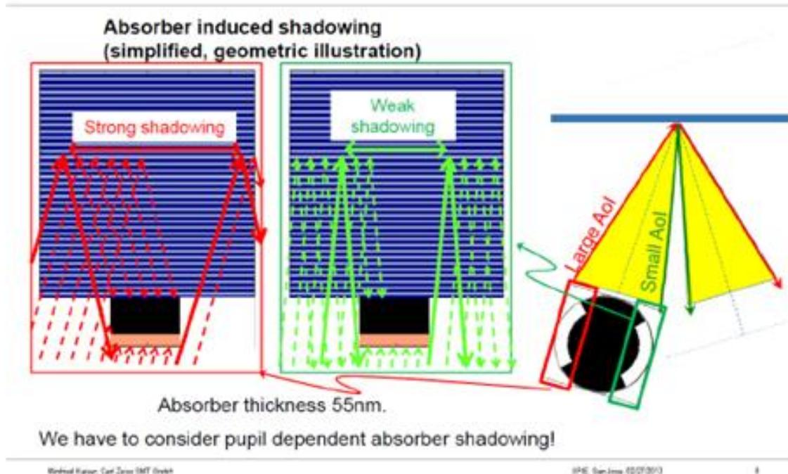
New mask structure including re-designed reflector and thin absorber is needed for high-NA system.
