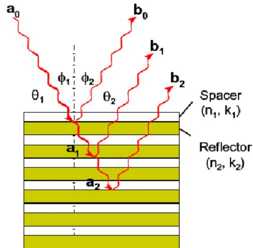
EUV Reflection by multilayer Bragg interference
